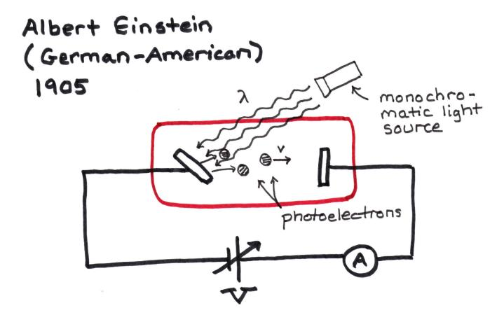
One photoelectron is liberated by one photon according to the conservation of energy equation
